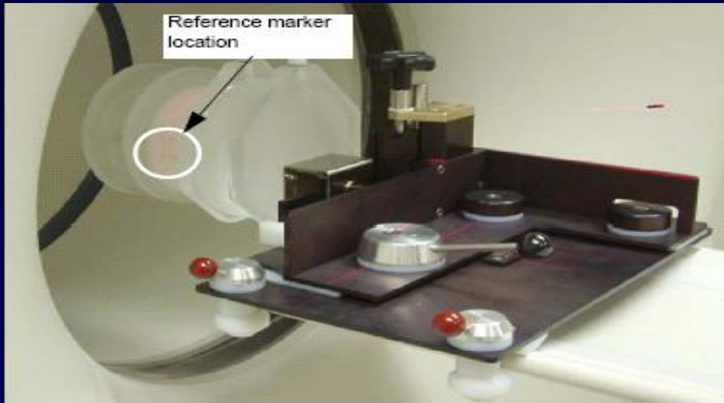
Figure 14: Slice-thickness phantom in position on the PHS, prior to moving PHS into CT gantry.
